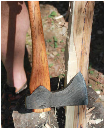
Using an axe to rough out the bow.
